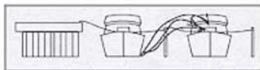
NEARBY BOAT GENERATOR EXHAUST
