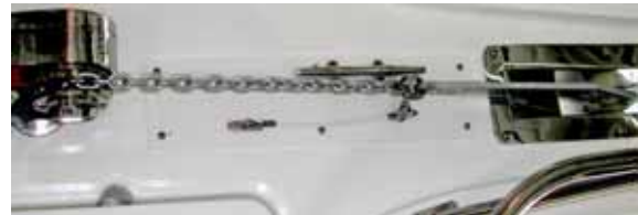
Anchor Chain Properly Secured For Travels
