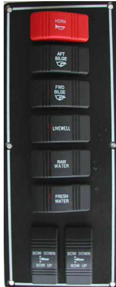
Helm Switch Panel Right
