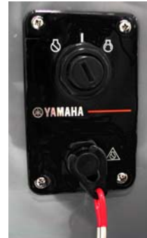
Engine Stop Switch
