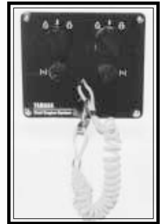
Engine Stop Switch
