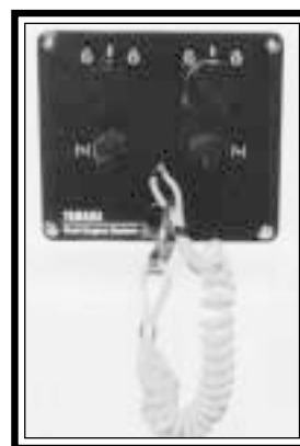
Engine Stop Switch
