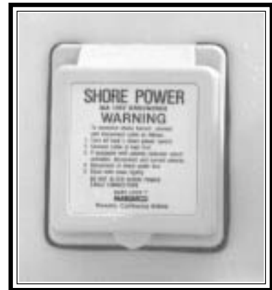
Shore Power Inlet
