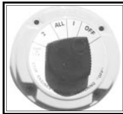
Battery Selector Switch
