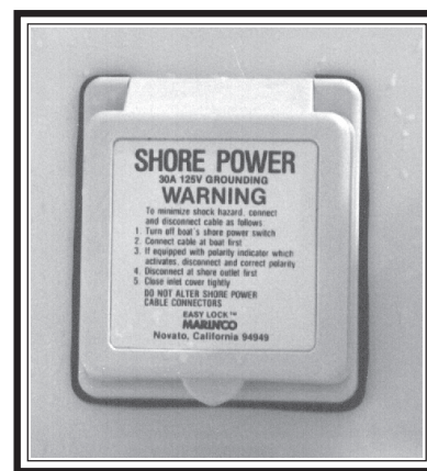
Shore Power Inlet
