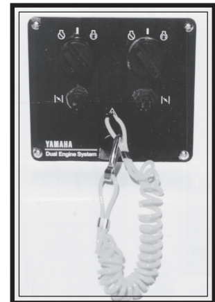
Engine Stop Switch
