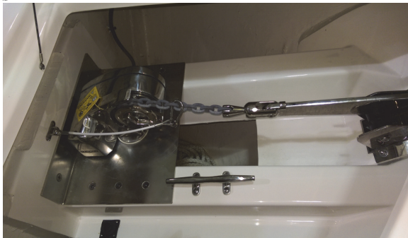
Anchor Line Secured Using Cable
