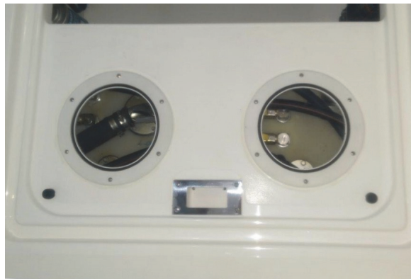
Gas Tank Valves
