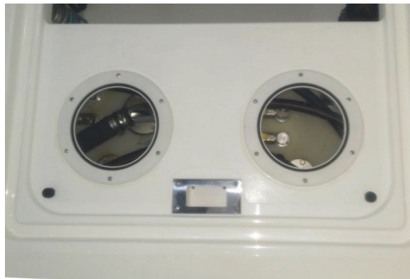
Gas Tank Valves
