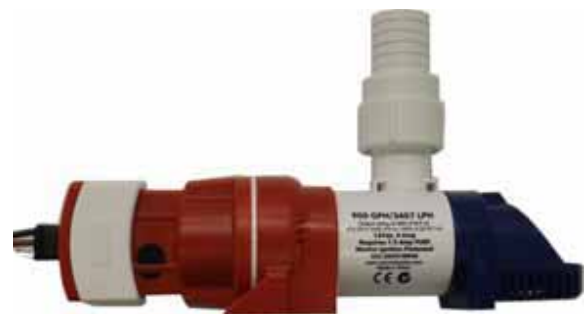
Aft Automatic Bilge Pump
