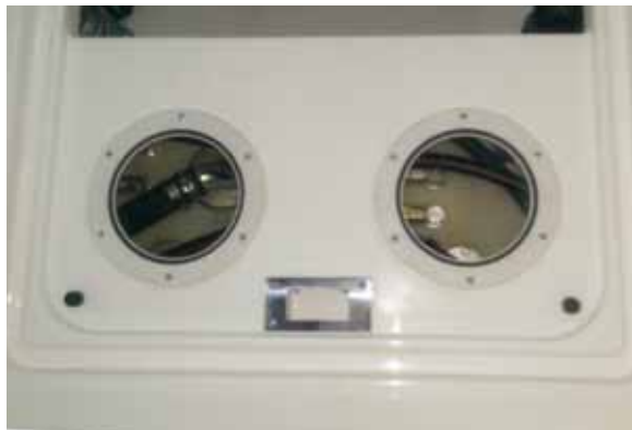
Gas Tank Valves
