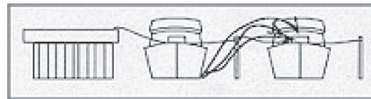
NEARBY BOAT GENERATOR EXHAUST
