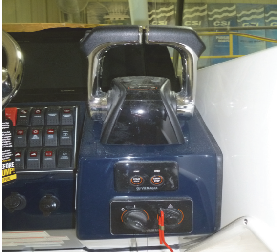
Engine Stop Switch
