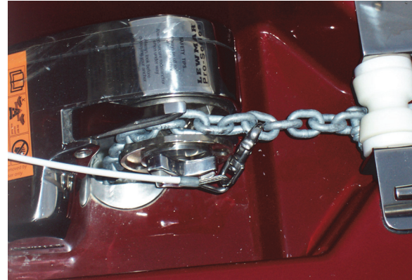
Anchor Chain Secured
