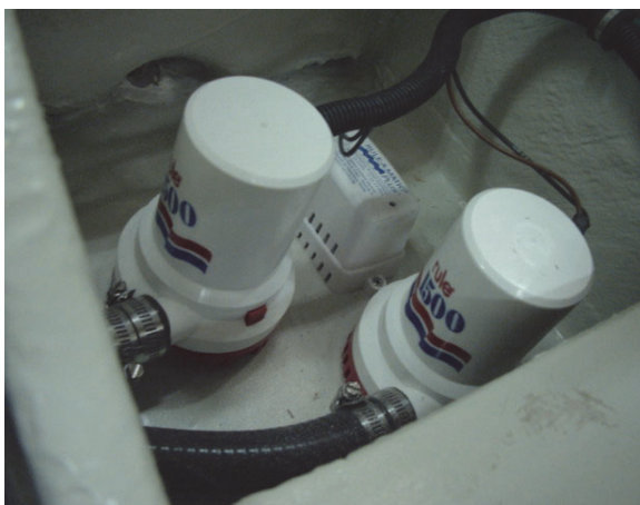
Bilge Pump (Typical)
