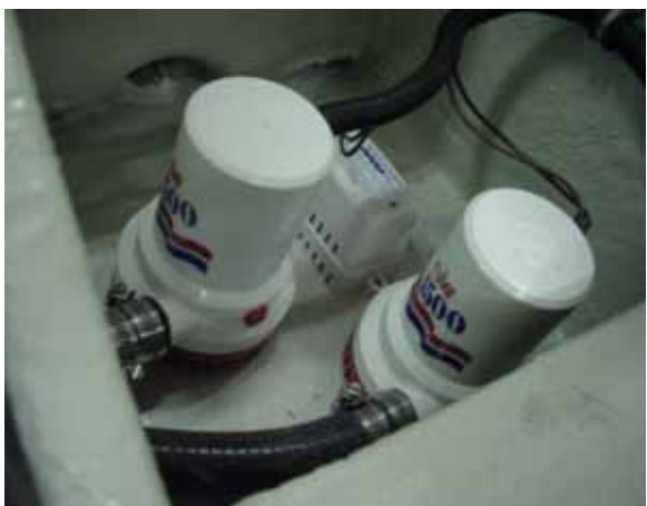
Bilge Pump (Typical)
