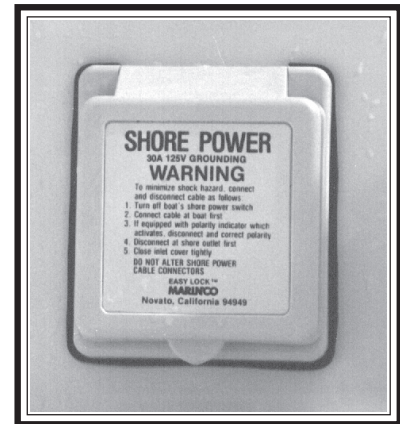
Shore Power Inlet
