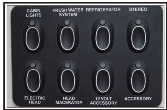
Cabin Switch Panel
