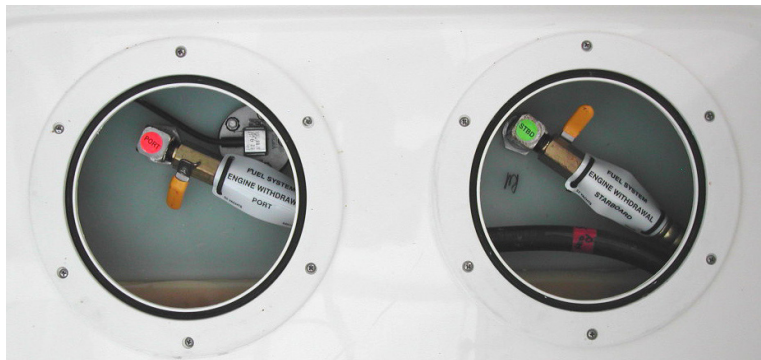
Fuel Valves Aft Tank
