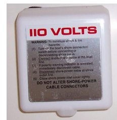
Shore Power Inlet
