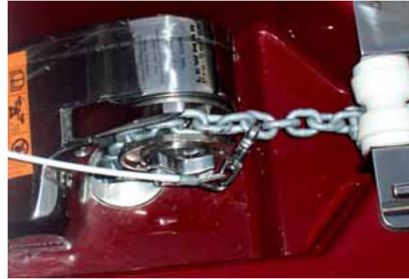
Anchor Chain Secured
