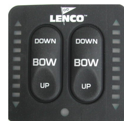
Trim Tab Switches
