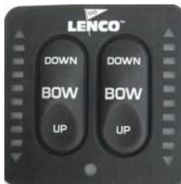
Trim Tab Switches
