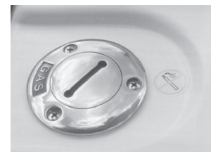
Fuel Fill (Typical)
