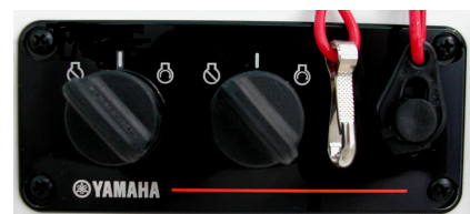
Engine Stop Switch
