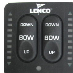
Trim Tab Switches
