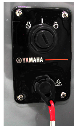
Engine Stop Switch
