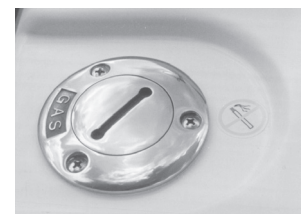
Fuel Fill (Typical)
