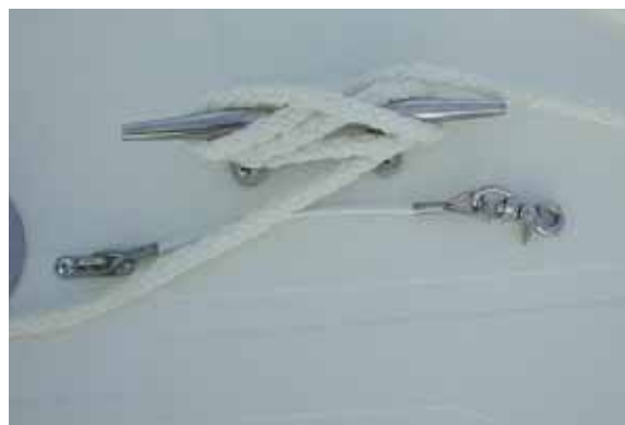
Anchor Line Secured to Cleat
