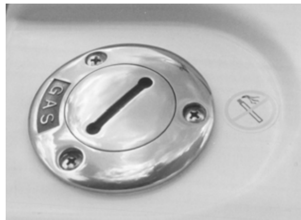
Fuel Fill (Typical)
