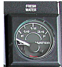
Fresh Water Tank Gauge
