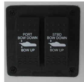
Trim Tab Switch Panel
