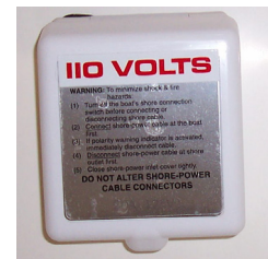
Shore Power Inlet
