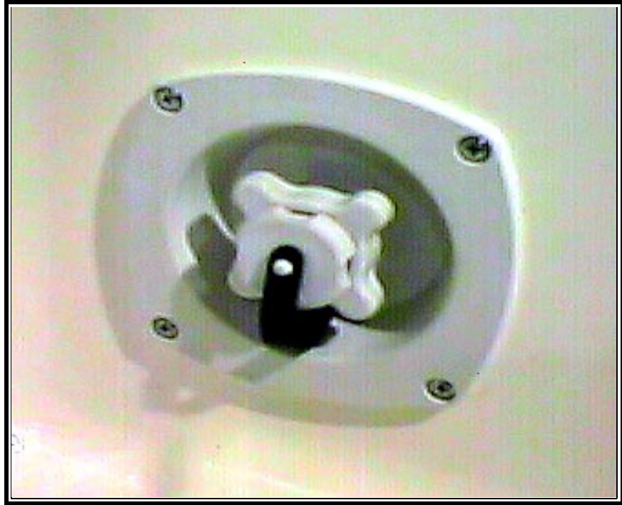
Figure 1-13: Dockside Water Inlet
