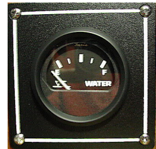
Fresh Water Tank Gauge
