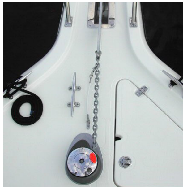
Anchor Chain Properly Secured For Travels
