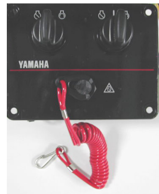
Engine Stop Switch
