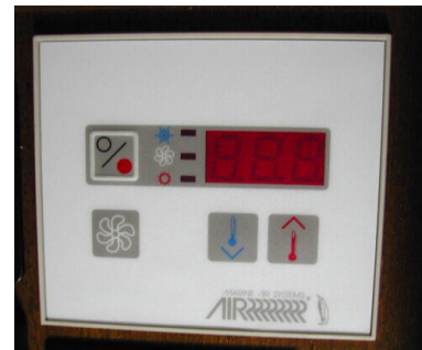
Air Conditioning Control Panel
