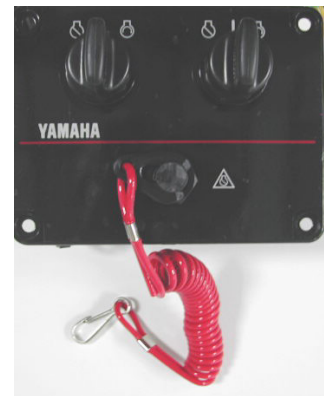
Engine Stop Switch
