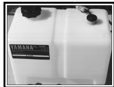
Engine Oil Tank
