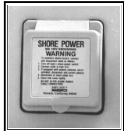
Shore Power Inlet
