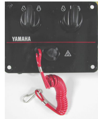
Engine Stop Switch
