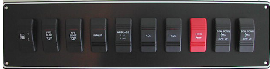
Lower Helm Switch Panel
