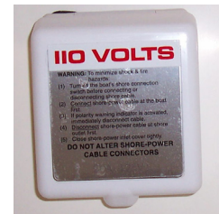
Shore Power Inlet
