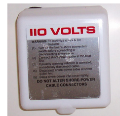
Shore Power Inlet
