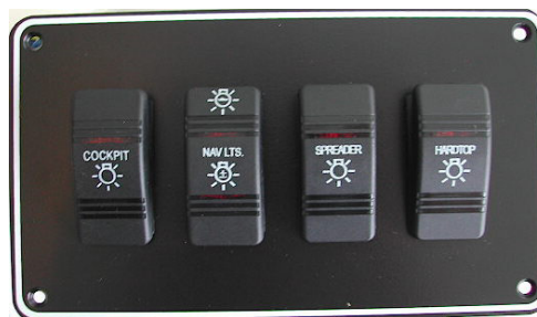
Upper Helm Switch Panel (Typical)
