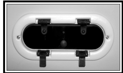
Opening Port Window
