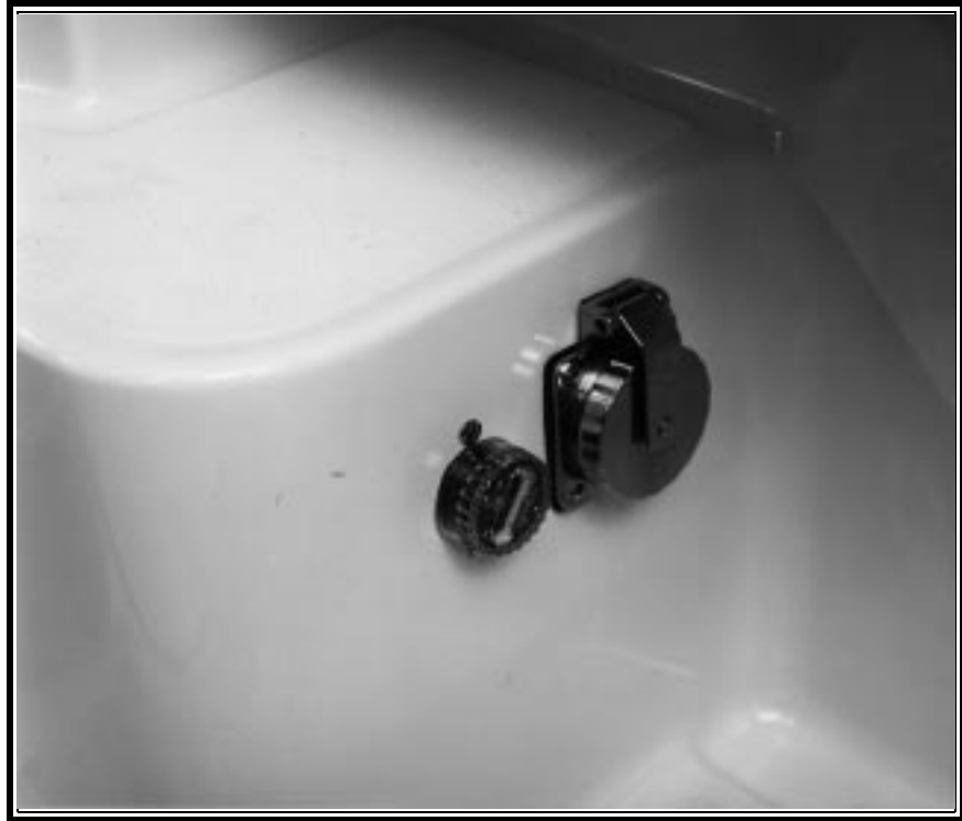
Figure 1-15: Shore Power Inlet
