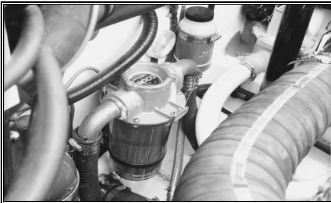
Figure 5-6: Engine Intake Pickup & Strainer
