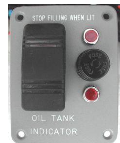
Oil Tank Indicator
