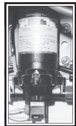
Fresh Water Pump
