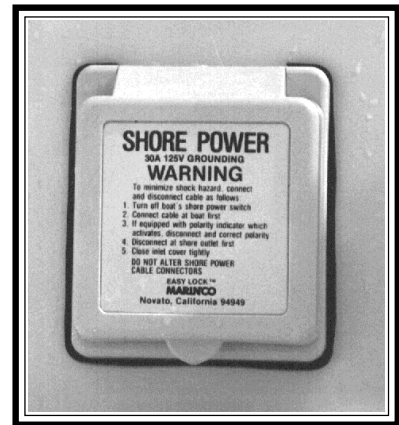
Shore Power Inlet
