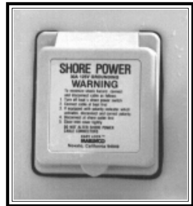
Shore Power Inlet
