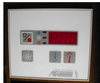
Air Conditioning Control Panel
