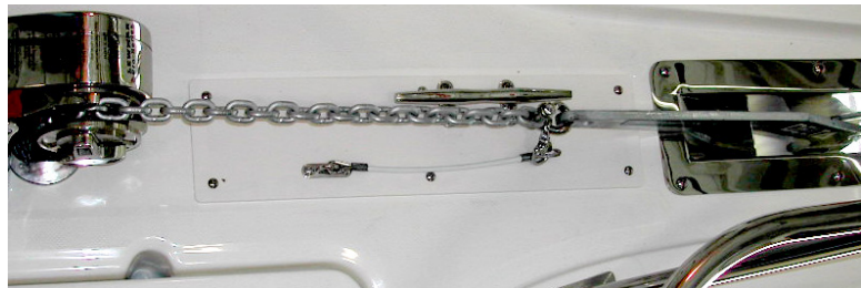
Anchor Chain Properly Secured For Travels
