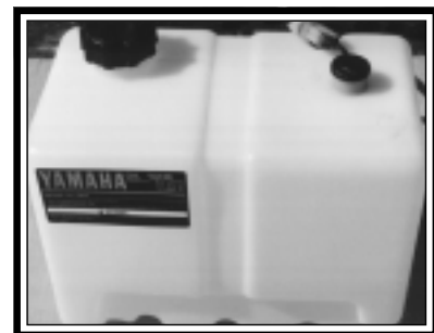
Engine Oil Tank
