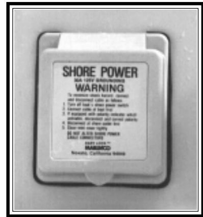
Shore Power Inlet
