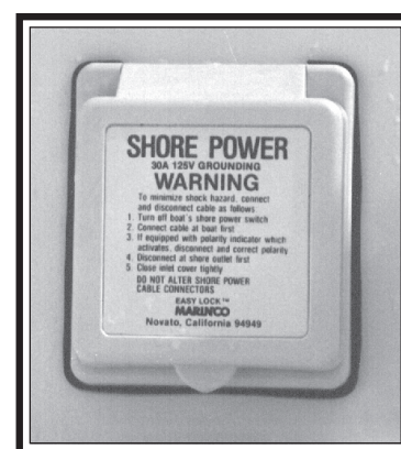
Shore Power Inlet
