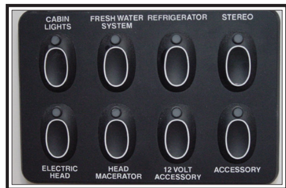
Cabin Switch Panel
