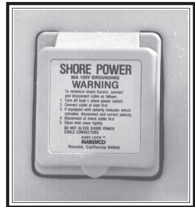
Shore Power Inlet
