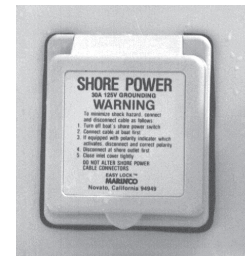
Shore Power Inlet
