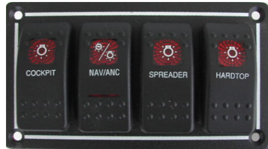
Left Helm Switch Panel
