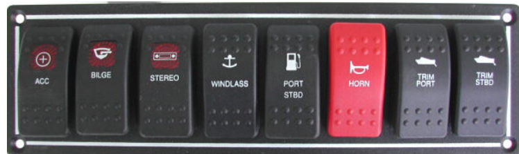
Right Helm Switch Panel
