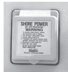
Shore Power Inlet
