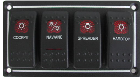
Upper Helm Switch Panel
