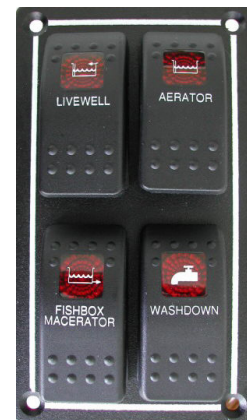
Cockpit Switch Panel
