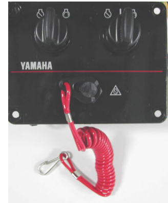
Engine Stop Switch
