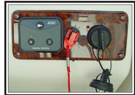
Engine Stop Switch
